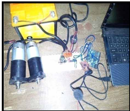
Complete circuit of the wheel chair
